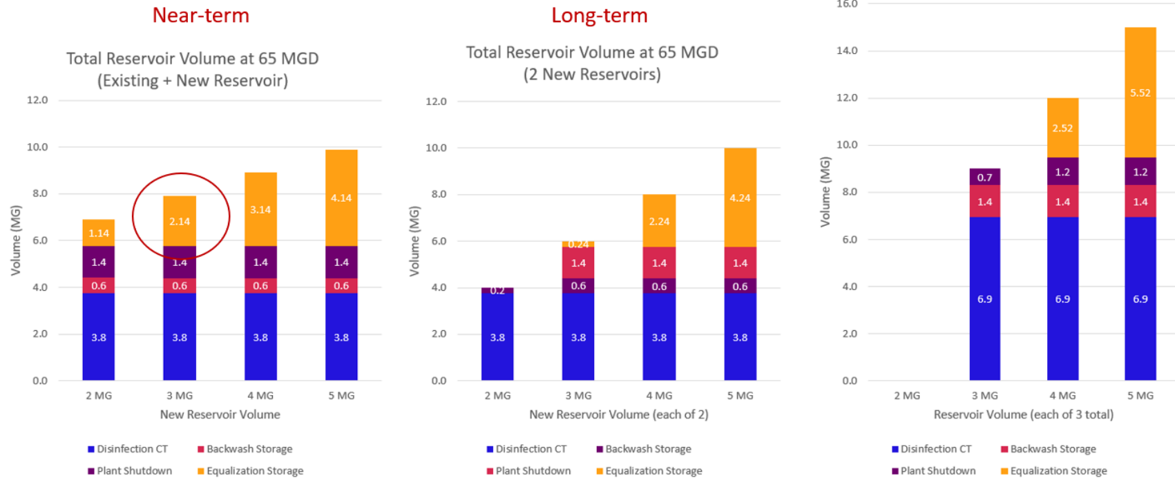
Figure 3.7 Duff Reservoir Equalizing Storage
